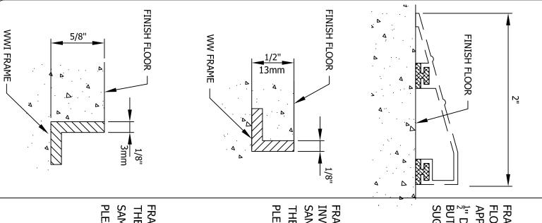
FRAME TYPE SSA = ALUMINUM AND COMES ABOVE THE FINISH FLOOR <u>WITHOUT DEPRESSION NEEDED</u> (SURFACE MOUNTED APPLICATION). THE WIDTH OF THE OVERLAP IS 2", IT BEGINS AT  $\frac{1}{2}$ " DEEP AND FINISHING AT "0" (BEVELED END) ON 4 CORNERS BUT IT'S AVAILABLE WITH 1, 2, 3 SIDES IF REQUESTED. WE SUGGEST TO ASSEMBLY ON SITE WITH A PL GLUE.
